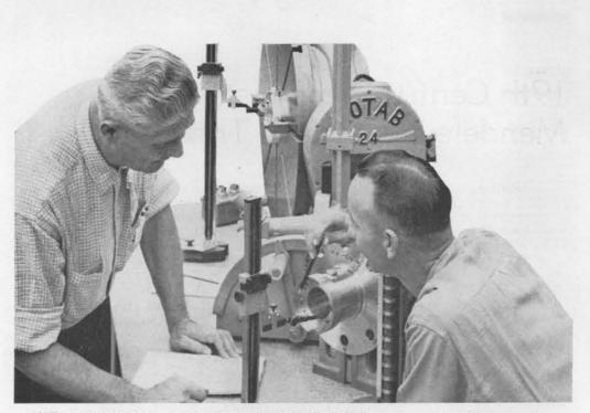
SAFETY ENGINEERING AND ENVIRONMENTAL HEALTH DIVISION 8242: Ray Campbell (8242-2), right, conducts test with air sampling device to determine amount of dust in air surrounding C. J. Tillman (8223-1) while machining material on lathe. Industrial hygiene, health physics, industrial accident prevention, fire prevention activities, and control of explosives, toxic, flammable, radioactive and special materials are also part of this division's job.
